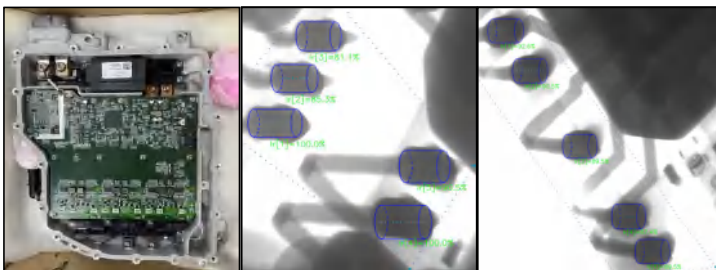
Inline Inspection of tin-penetration of automotive power modules
